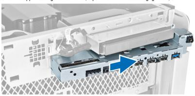
7. Remove the screws that secure the USB 3.0 module to the front I/O panel and remove it from the computer.
