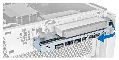
6. Slide the opposite edge of the front I/O panel outward to disengage the I/O module from the chassis.
