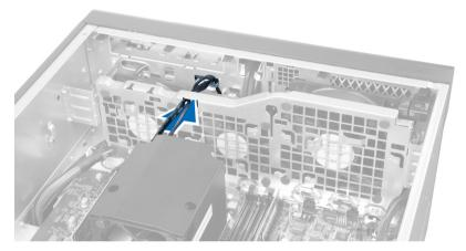
10. Disconnect the system fan cable connectors from the system board.
