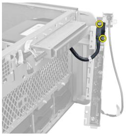
8. Remove the screws that secure the front I/O panel and remove it from the computer.
