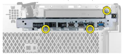
5. Pull the front I/O panel in a direction opposite to the computer to release its edge from the chassis clip.
