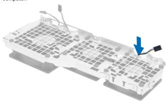
13. Remove the rubber tabs that secure the system fan , lift up the fan and remove it from the fan assembly.
