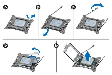
4. Repeat the above steps to remove the second processor (if available) from the computer. To verify if your computer has dual processor slots, see the System Board Components.
