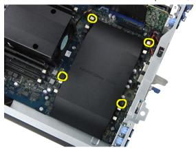
**4.** Remove the processor/memory slot cover from the computer.
