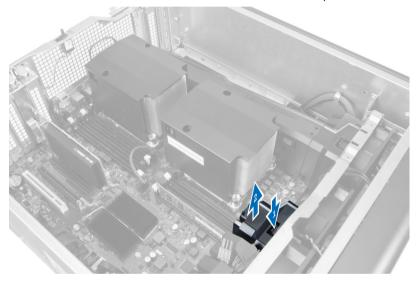
**6.** Repeat the steps to remove the second air tunnel module from the computer.
