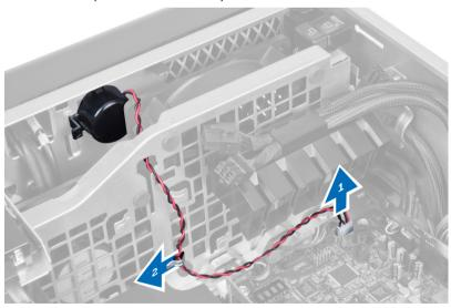
3. Press the speaker latch on both sides to release the speaker from the chassis and remove it from the computer.
