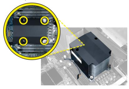
5. Lift up the heat sink and remove it from the computer.
