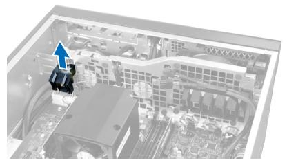
6. Slide the second air duct in the direction of the system fan to loosen it from its retention clasps.
