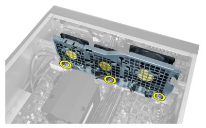
**12.** Disconnect the system-fan cable from the system fan module and remove the system fan module from the computer.
